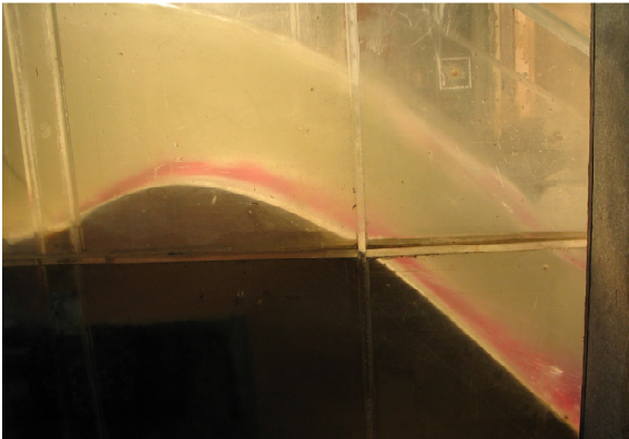
Figure 5a: The streamlines along the spillway.
