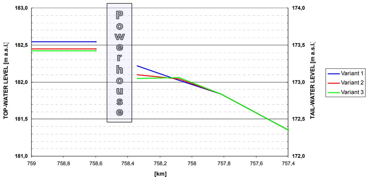
Fig. 4: The Water Level Profile for the Different Variants
