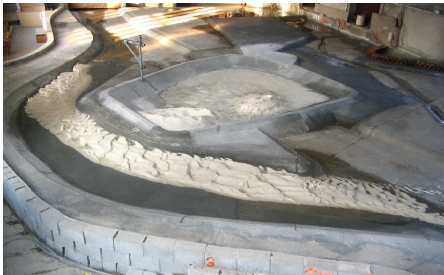
Figure 7. Strong erosion on the concave part of the diversion channel after 27 hours of operation at the flow Q = 1800 \text{ m}^3/\text{s} .
