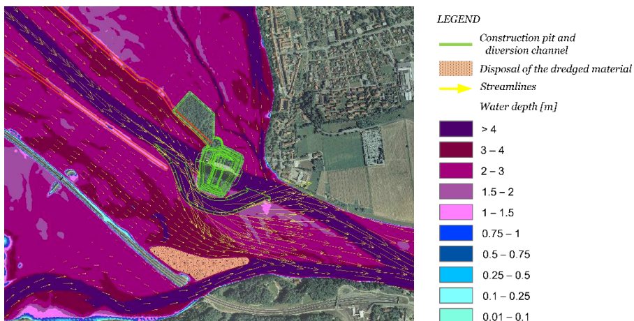
Figure 11. Final location and shape of the disposal site for excavated material from the construction pit and diversion channel, showing the velocity field at 100 year return period event.
