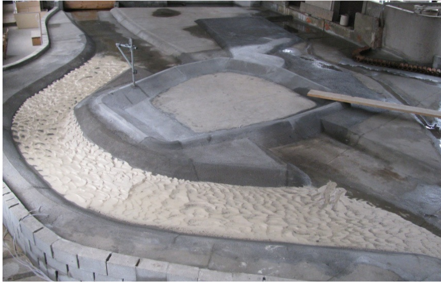
Figure 6. The bottom of the diversion channel on the physical model after 11.7 hours at the flow Q = 500 \text{ m}^3/\text{s} .
