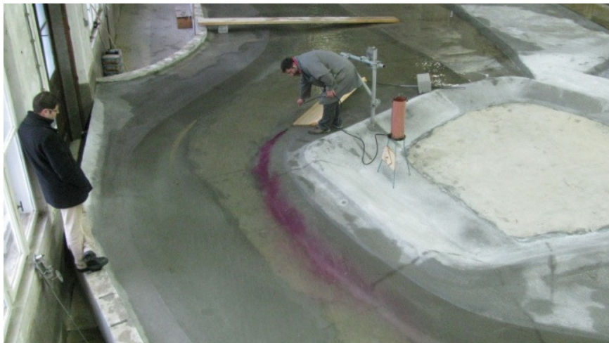
Figure 4. Streamlines along the construction pit with an optimized narrower inflow into the diversion channel. A smaller calm zone appears along the construction pit with less prominent vortices at the edge of the pit. The extent of the excavation is also smaller.
