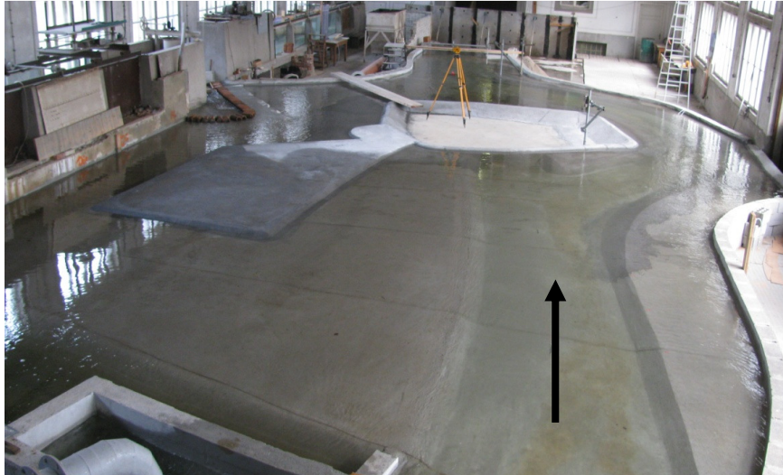
Figure 2. Physical hydraulic model of the HPP Brežice including the construction pit and the diversion channel.
