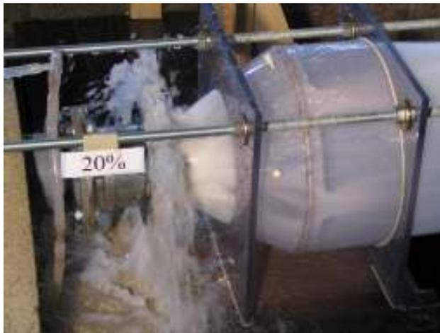
Fig. 4: Valve moved 10 cm downstream,  $s = 20\%$ .
