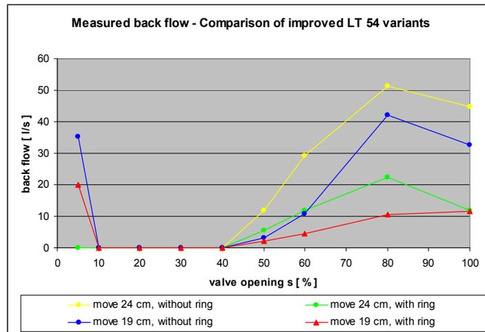
Fig. 7: Some results of the back splash measurements show significant influence of the additional ring.
