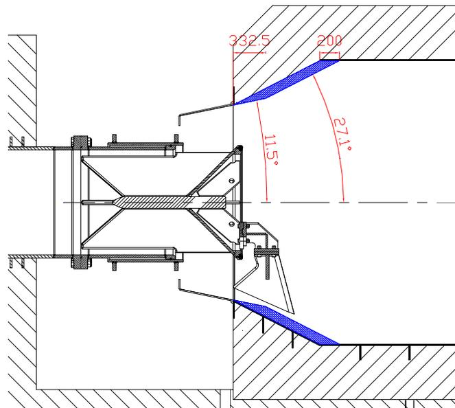
Fig. 8: The longitudinal section of the final solution (in mm): The combination of LT 54, ring and hood modification.
