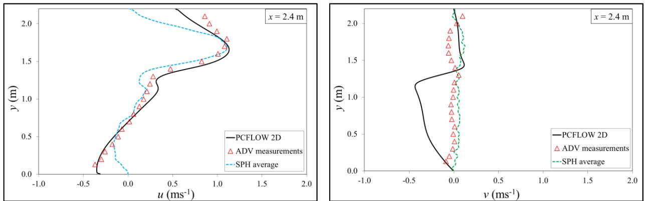
**Figure 10.** Average velocity profiles at location  $x = 2.4$  m.
