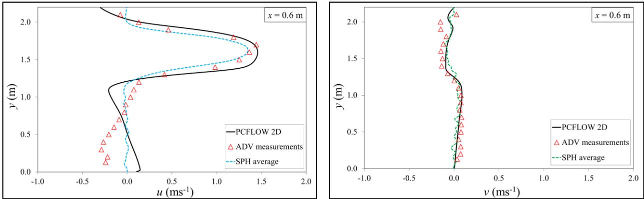
Figure 7. Average velocity profiles at location  $x = 0.6$  m.
