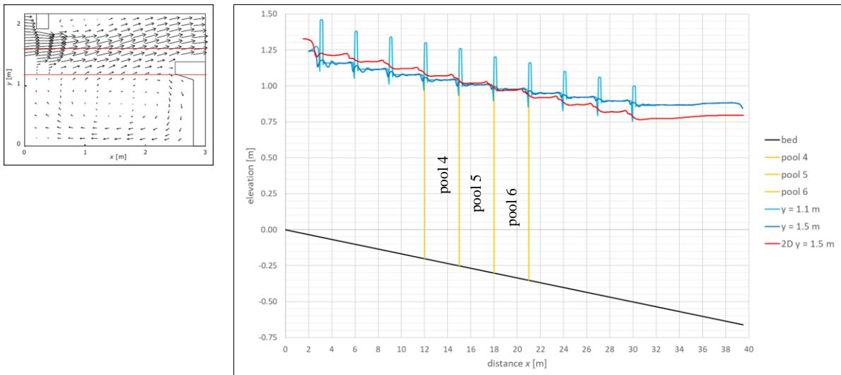
**Figure 4.** Longitudinal water surface elevation profiles along the  $y = 1.1$  m line and along the  $y = 1.5$  m line (see the top left frame). Results of the 2D model are in red, Dual SPHysics v4.2 results are in blue.
