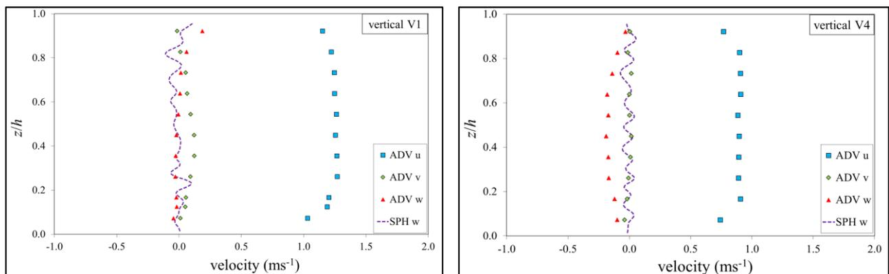
**Figure 5.** Vertical distribution of the velocity components in the main flow region.
