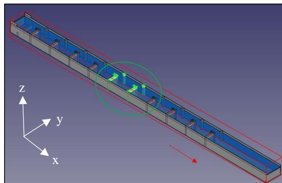
**Figure 2.** The geometry of the VSF, with observed middle pool (in green) and flow direction (red arrow).
