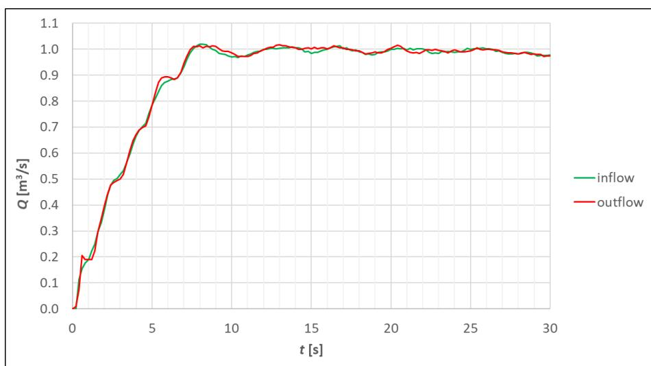
Figure 3. Inflow to and outflow out of the observed pool in Dual SPHysics v4.2.
