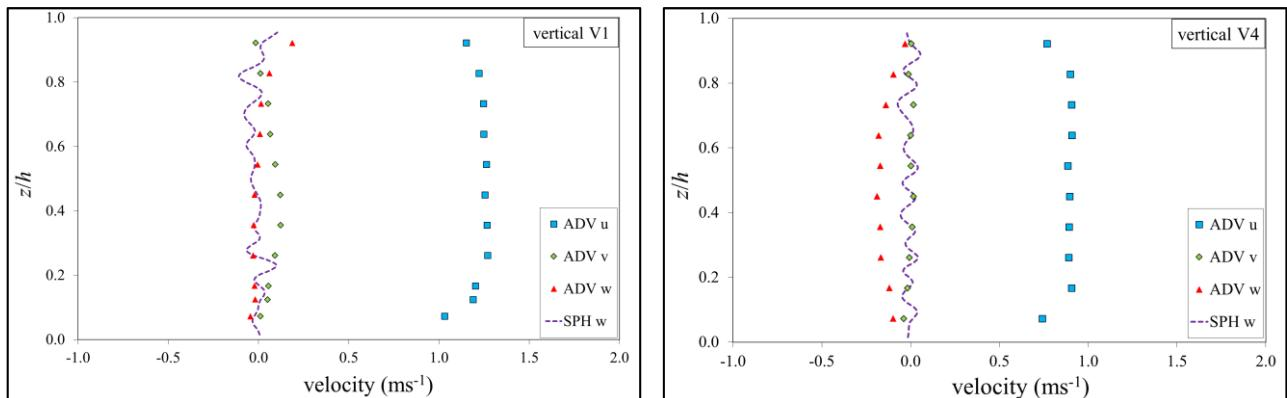
**Figure 5.** Vertical distribution of the velocity components in the main flow region.
