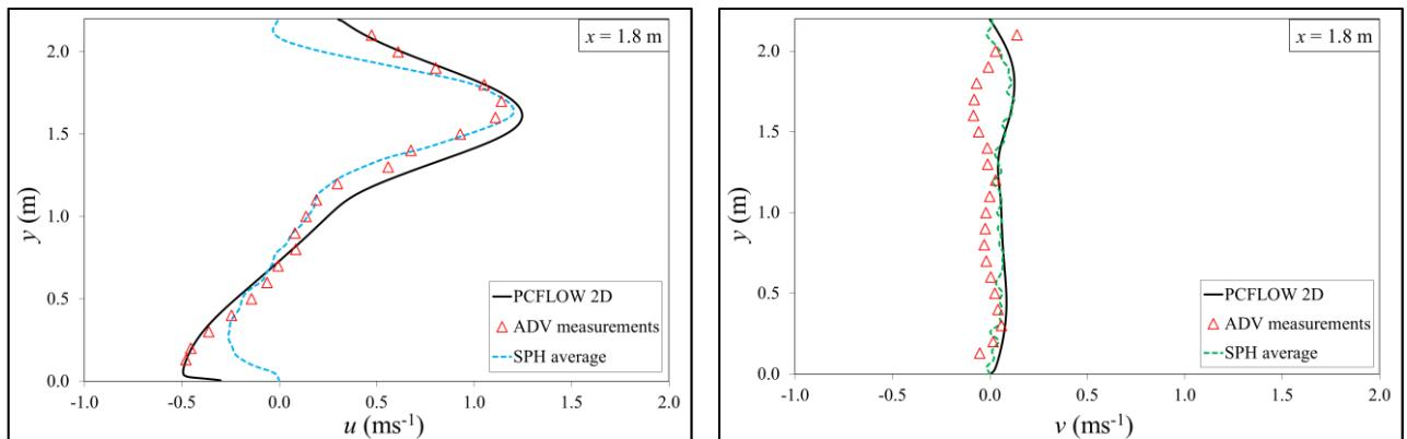
**Figure 9.** Average velocity profiles at location  $x = 1.8$  m.
