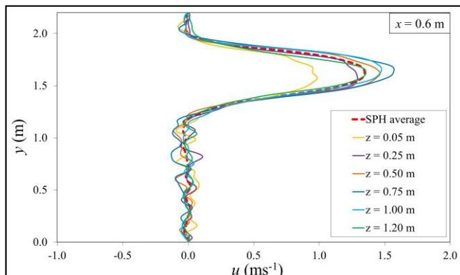
**Figure 6.** Calculation of average profile of velocity  $u$  at location  $x = 0.6$  m.
